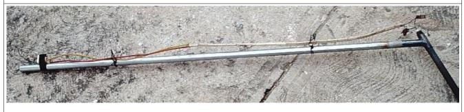
I cut a shallow groove in the top of the graphite sheath to wrap a piece of wire in to keep the sheath from slipping out of the tube.
