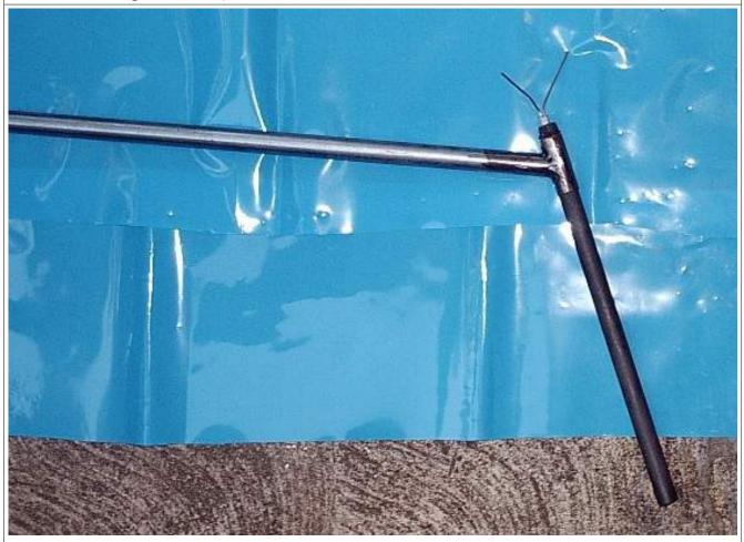
I ran the extension wires in ceramic insulators down to the end of the handle. If you use fiberglass insulated wire it will be fine without the insulators.
