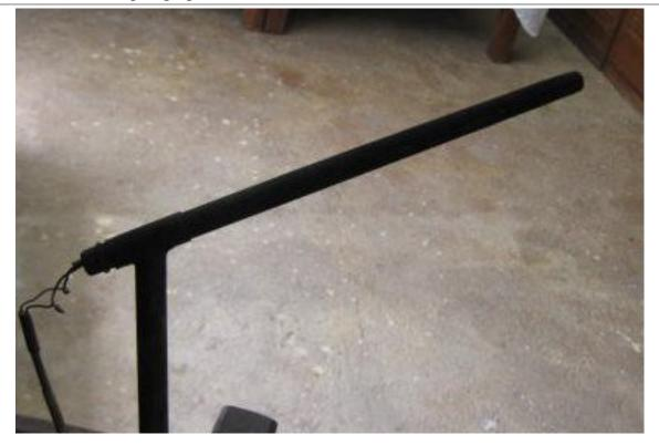
While I was set up I drilled all five rods which should last me for several years in my occasional use. I am a sculptor and melt bronze maybe three times a month. One advantage of these over the Mifco Inconel probes is that molten metal just slides off of the graphite; you don't have to scrape them after use.
